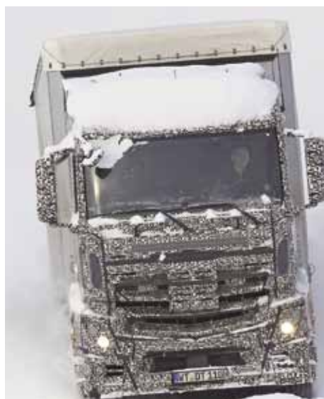
A Mercedes-Benz Actros (still in camouflage) undergoing winter testing to -40°C in Rovaniemi, Finland. The company tests many of its industrial engines in trucks like this
