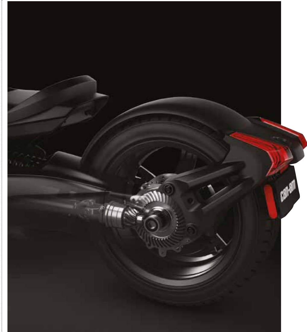
A mechanical final drive was chosen over a belt due to the distance from the engine
